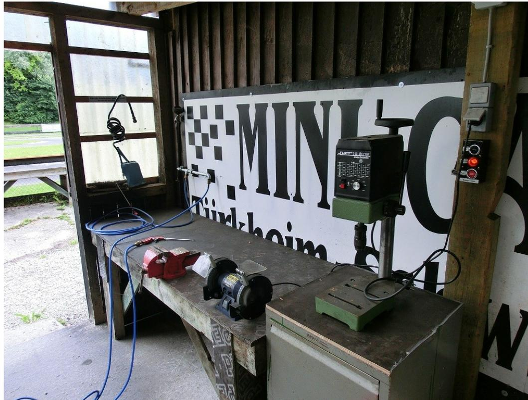
The place for truing tires has also a workbench with "big" tools like a pillar drill, a bench grinder and a bench vise.
